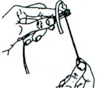
Thread tag end of line into groove under wraps starting at thumb and proceeding toward tip of tool.
